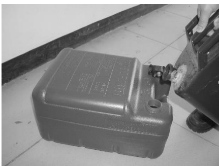
External fuel tank
