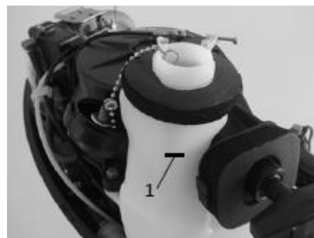
Internal fuel tank
