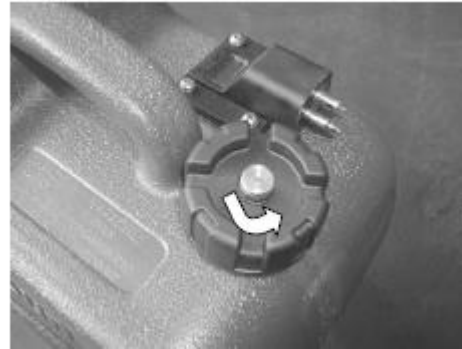
External fuel tank
