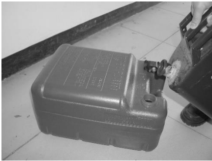
External fuel tank
